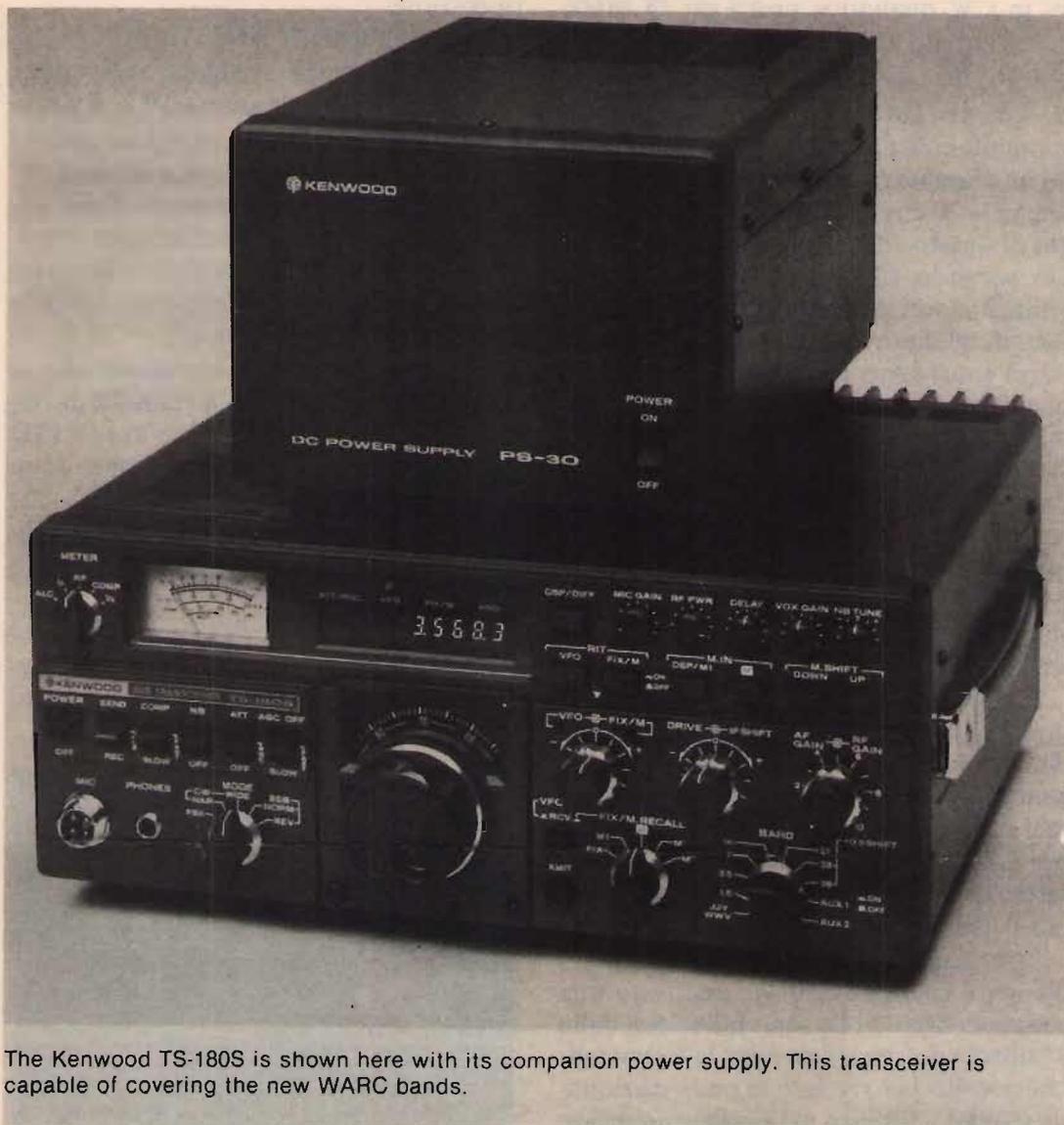
The Kenwood TS-180S is shown here with its companion power supply. This transceiver is capable of covering the new WARC bands.
